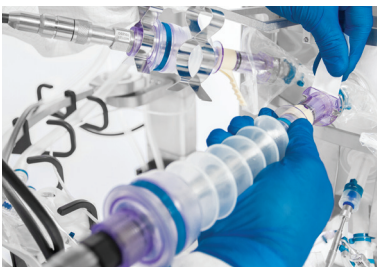
Figure 6. Bioreactor probe assembly.
