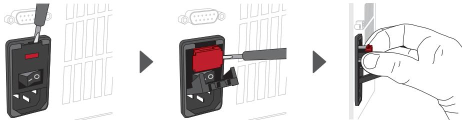
4. Remove each fuse from its fuse holder, then inspect it for damage.
