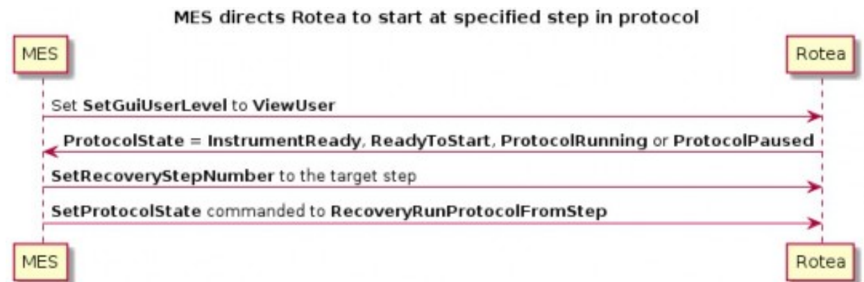
Figure 17 Perform run from step recovery operations from OPC-UA while running a protocol
