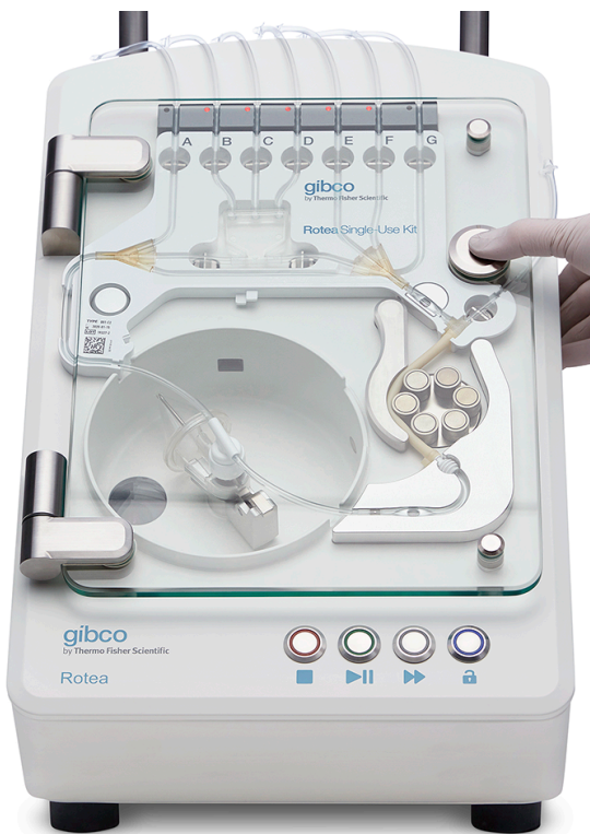
Figure 6 Instrument with CTS™ Rotea™ Single-Use Kit
