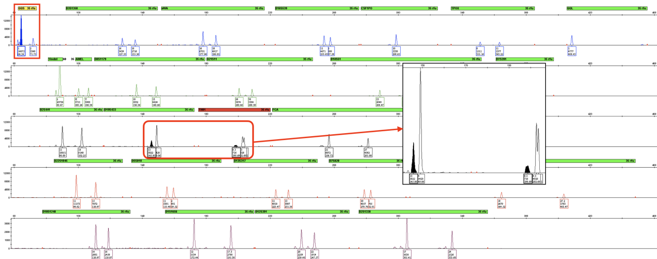
Figure 46 Potential artifacts seen in the NED™ dye channel at D19S433 and TH01 when sample loads are excessive. The QQS 1 peak is >3,800 RFU and the QTS value in RapidLINK™ Software v2.0 is >2 ng. D19S433 displays extremely high stutter (30–45%) and TH01 shows a peak 5 bp in front of a main allele peak. The inset shows a closer view of the D19S433 and TH01 artifact peaks circled in red. The QQS loci (outlined by the red rectangle in the FAM™ dye channel) shows a QQS 1 quantification peak of 14,875, an estimated sample load of 7.85 ng.
