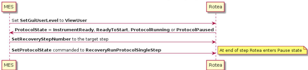
Figure 8 Performing single step recovery operation from OPC-UA while running a protocol
