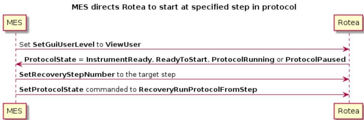
Figure 9 Performing run from step recovery operations from OPC-UA while running a protocol
