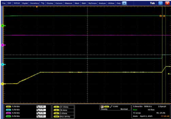
Figure 5. Power-up slew rate, programmed to 1 msec using MK.4TE Scimitar Software and the high-current power supply option.
