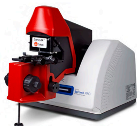
Figure 4. Nicolet Summit FTIR Spectrometer with the SurveyIR® Accessory in the sample compartment.
