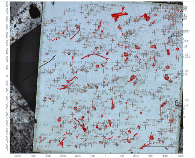
Figure 2. A silicon filter with atmospheric deposition of microplastics. Particles selected are between the size range of 25 \mu\text{m} – 1 mm.
